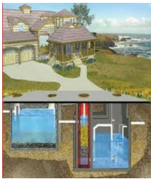
Figure 1. Illustration of the Amphidrome® sequencing batch reactor as configured for testing at the Massachusetts Alternative Septic System Test Center.
